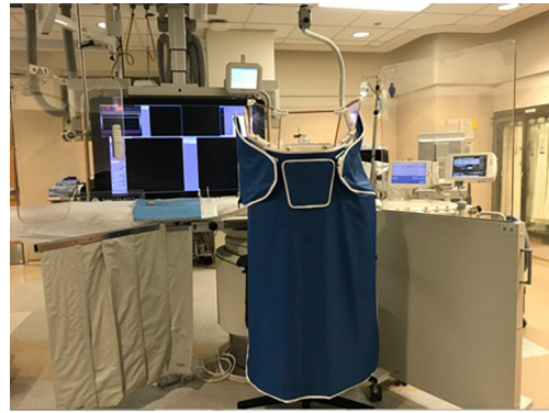
Figure 1 Radiation protection equipment in a modern cardiac catheterization laboratory. In this picture you will find ceiling-mounted lead glass shield, under-table lead curtain, radioabsorbent patient drape, real-time radiation dose monitor, Zero-gravity system, and a rolling lead shield.
