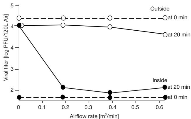
**Figure 4** Viral titers in the sampled air collected inside and outside the positive-pressure hood at 0 and 20 min after atomization of the viral fluid outside the hood under active FFU with various airflow rates. Open circle, outside the hood; solid circle, inside the hood. Solid line, 20 min; broken line 0 min. FFU, fan-filter-unit.
