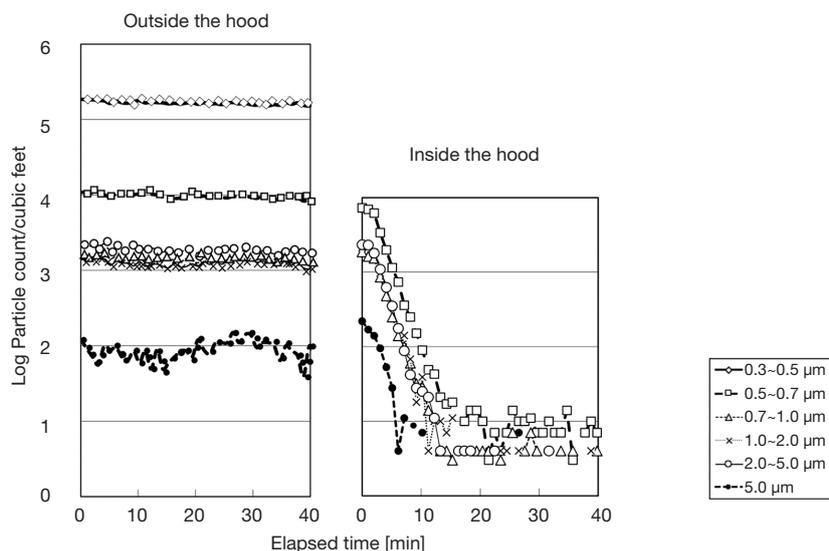
**Figure 2** Concentration of airborne particles with size greater than  $0.3 \mu\text{m}$ , inside and outside the positive-pressure hood with the FFU switched on with airflow rate  $0.19 \text{ m}^3/\text{min}$ . Saline was atomized outside the hood and airborne particle concentrations of the air inside and outside the hood were measured at several time intervals after the atomization.
