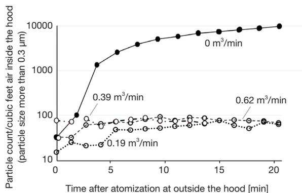
**Figure 3** Time course of concentration of airborne particles of various sizes of saline mist inside the hood after atomization at the outside under active fan-filter-unit (FFU) with various airflow rates,  $0.42 \text{ m}^3/\text{min}$ .
